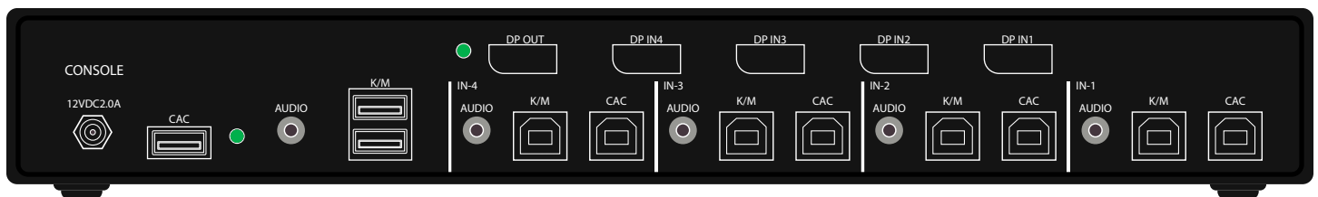
Figure 4-2: SA-DPN-4S-P Rear panel
