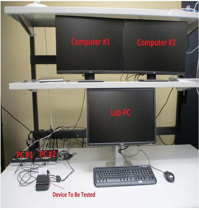
The photograph above shows the environment where the device will be tested. The evaluator used two test computers (Computer #1 and #2) as well as a Lab PC. The device being tested was connected to one or both computers, as well as the lab PC to conduct testing.
