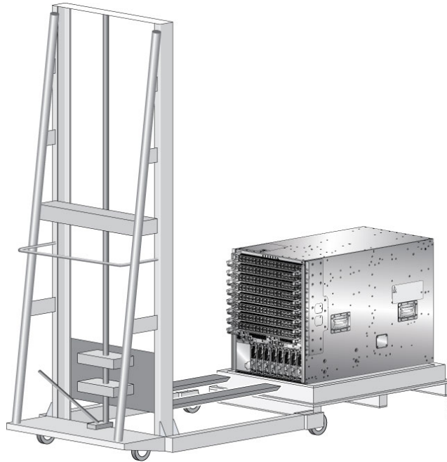
Figure 12: Align the Lifting Device in Front of the Chassis on the Pallet
