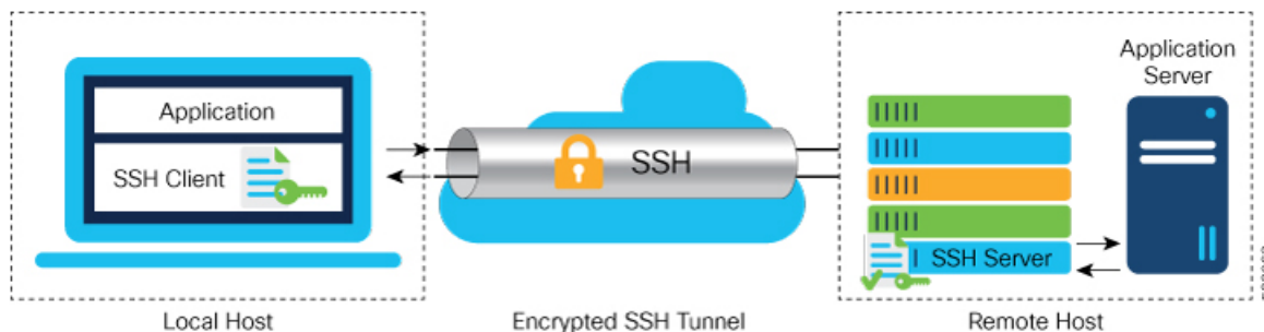
Figure 11: SSH Port Forwarding
