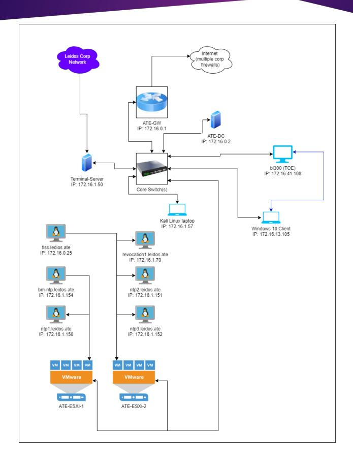
Note: The blue connection between the Windows 10 client and the BL300 (TOE) represents the physical serial connection that is used for local connection/configuration.
