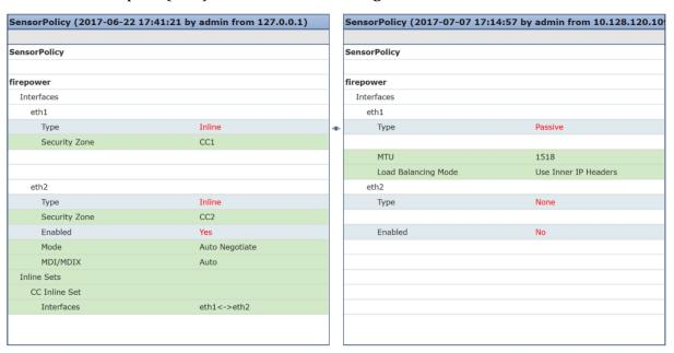
Note: eth1 and eth2 used to be inline and now eth1 is passive and eth2 is not active (i.e., disabled).
