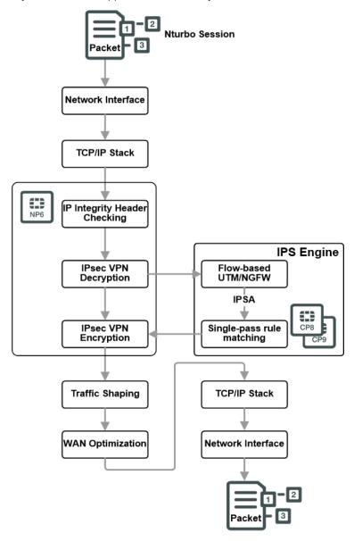
After the first packet, subsequent packets in an offloaded flow-based UTM/NGFW session skip routing, and kernel processors. Flow-based UTM/NGFW operations are still handled by the CPU with IPSA offloading pattern matching to CP8 or CP9 processors.
