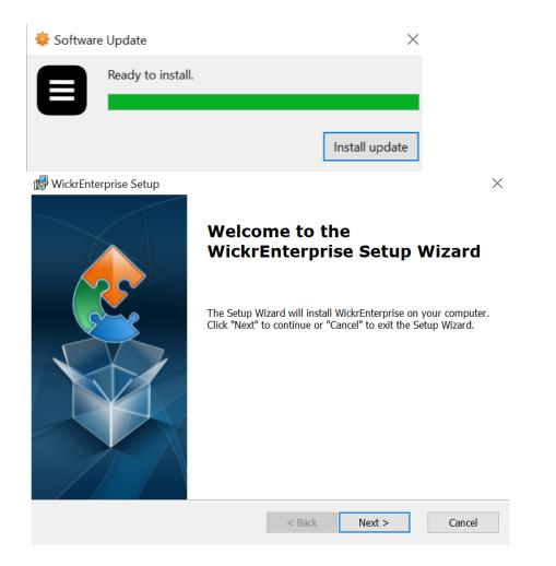
When an installation package is downloaded by the platform, it is verified prior to installation. Updates for the Android and Linux platform versions of the TOE are digitally signed using a 4096-bit RSA key; updates for the iOS, macOS and Windows platform versions of the TOE are digitally signed using a 2048-bit RSA key. Signature verification is performed automatically before proceeding with the package install. If the signature verification fails, the package is not installed.
