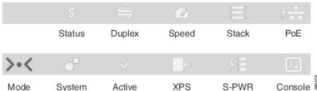
Figure 8: Switch Front Panel LEDs
