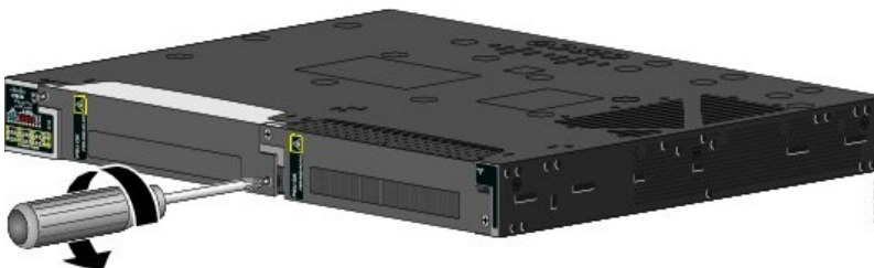
Figure 26: Loosening the Screws on the Power-Supply Blank
