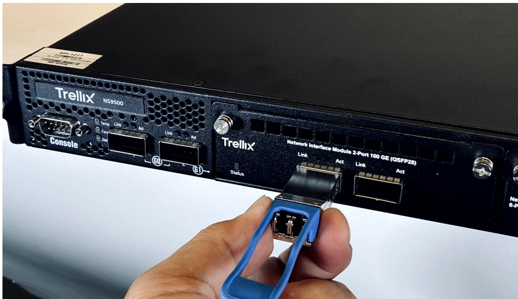
Insert a transceiver module
