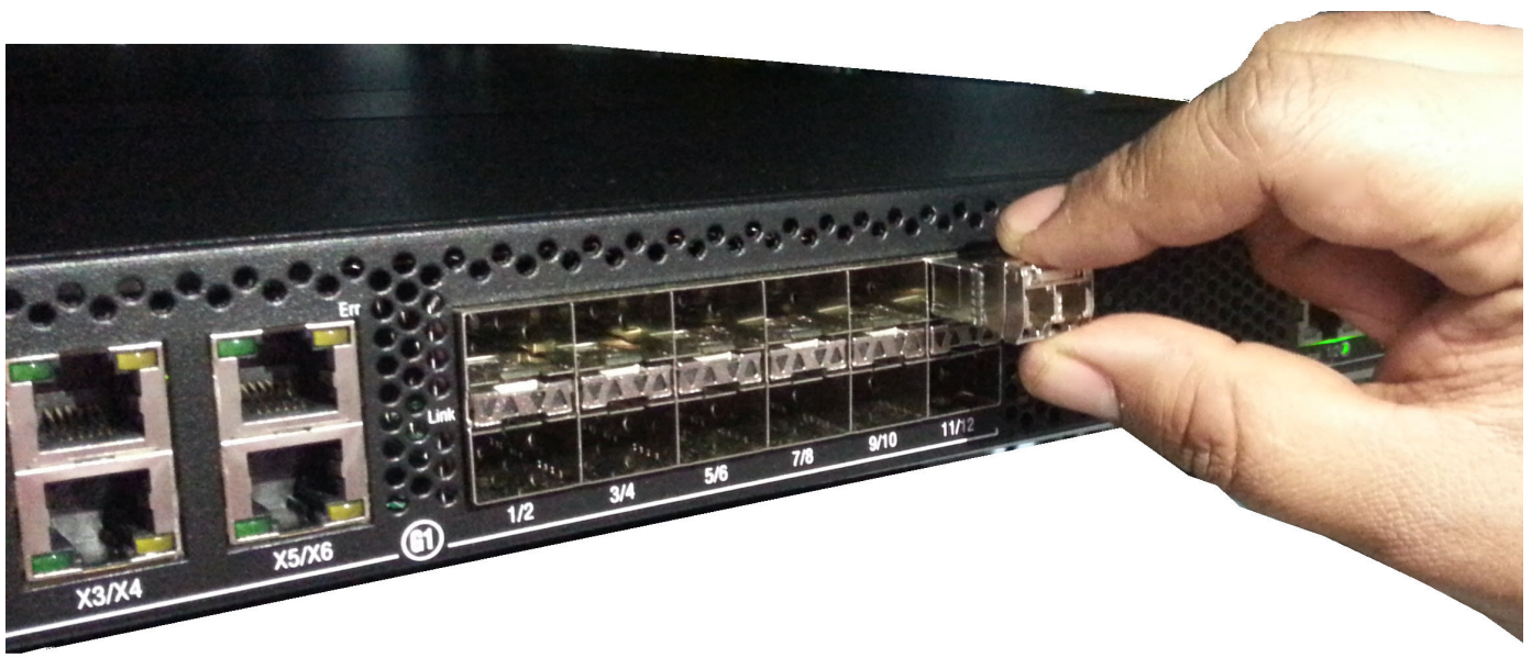
Insert a transceiver module
