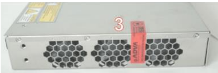
Figure 38: SH1HU-HP/2DC and SH1HU-HP/E-TEMP/2DC Right Side — Seal Locations
