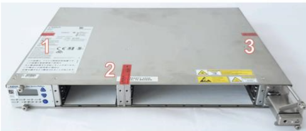
Figure 39: SH1HU-R/PF Front-Top View — Seal Locations
