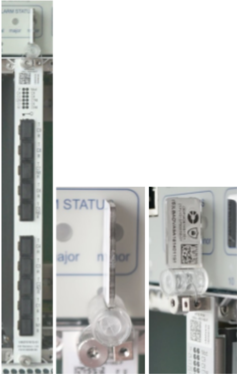
Figure 87: 9TCE-PCN-10GU+AES10G-F — Seal Locations
