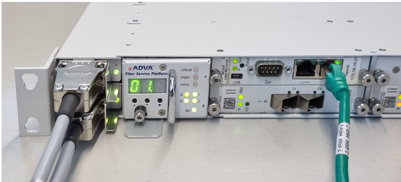
Figure 84: FAN/1HU-F Mounted in a SH1HU-F/E+TEMP/PF
