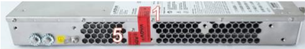
Figure 42: SH1HU-R/PF Viewed From Right Side — Seal Locations
