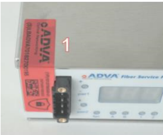
Figure 37: SH1HU-HP/2DC and SH1HU-HP/E-TEMP/2DC Top Front Side — Seal Locations
