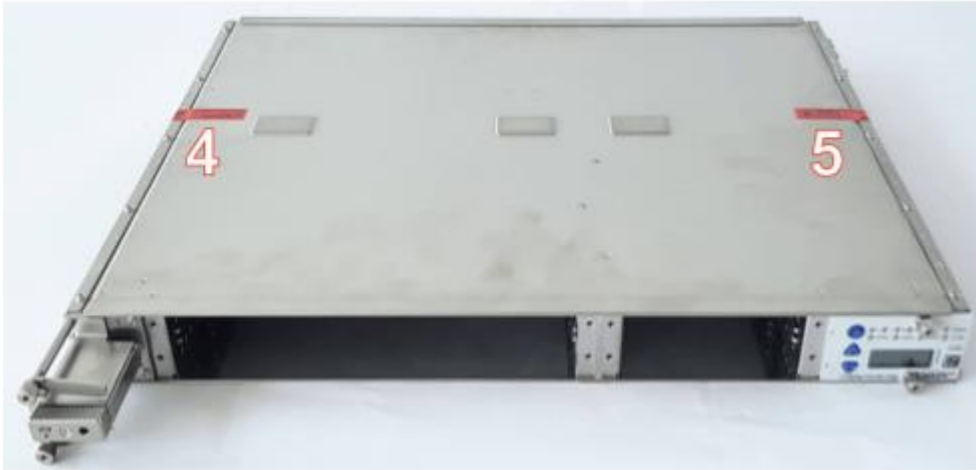
Figure 41: SH1HU-R/PF Viewed From Left Side — Seal Locations
