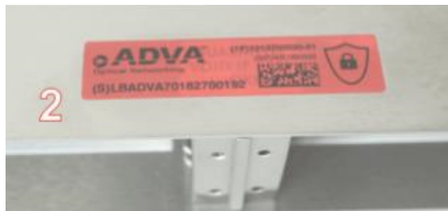
Figure 38: SH1HU-HP/2DC and SH1HU-HP/E-TEMP/2DC Right Side — Seal Locations
