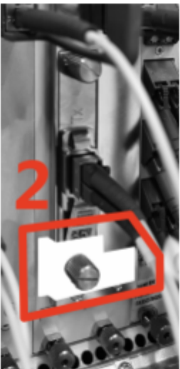
Figure 89: SEAL/FIPS-CFP Seal Label on the WCC-PCN-AES100G-F — Seal Location
