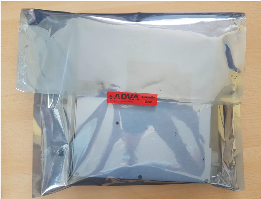
Figure 4: Tamper-Evident Seal Security Label on the ESD Protective Bag for a Shelf
