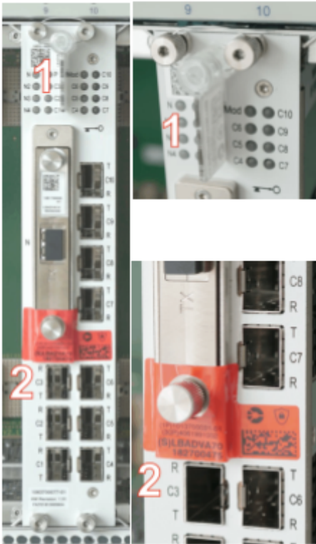
Figure 86: 10TCE-PCN-16GU+AES100G-F — Seal Locations
