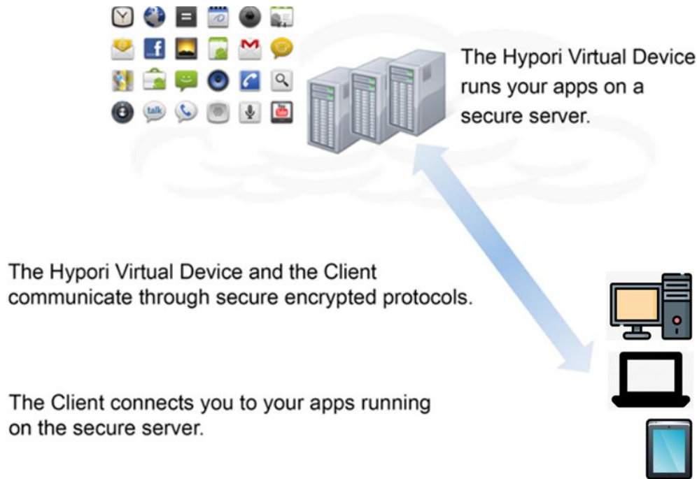
Figure 3 Hypori Halo Client Communication with a Hypori Virtual Device on a Hypori Server
