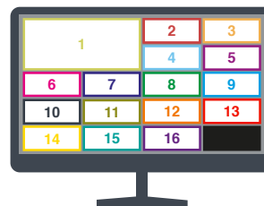
16 Ports Scale Layout Single/Clone display – in Extended mode the primary display will show one channel in Full layout and the secondary in will show the other 15 in Quad
