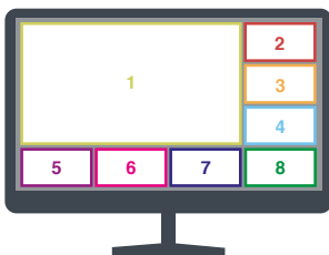
8 Ports Scale Layout Single/Clone display – in Extended mode the primary display will show one channel in Full layout and the secondary in will show the other 7 in Quad
